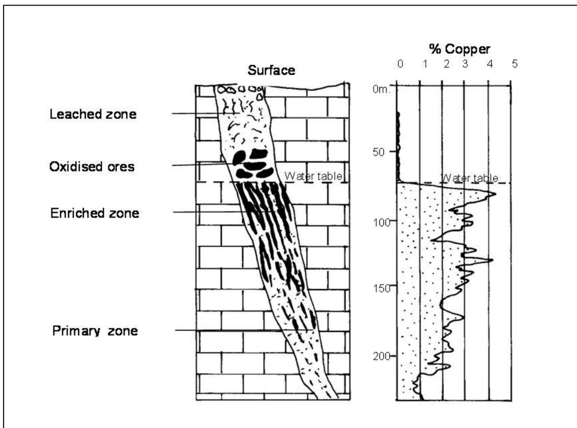
**Fig 3.4 A generalised section through a copper-bearing ore body.**
