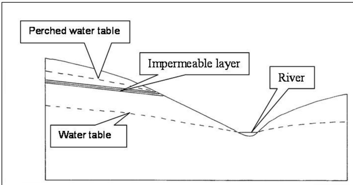
Fig 3.1 Diagrammatic section of the water table
