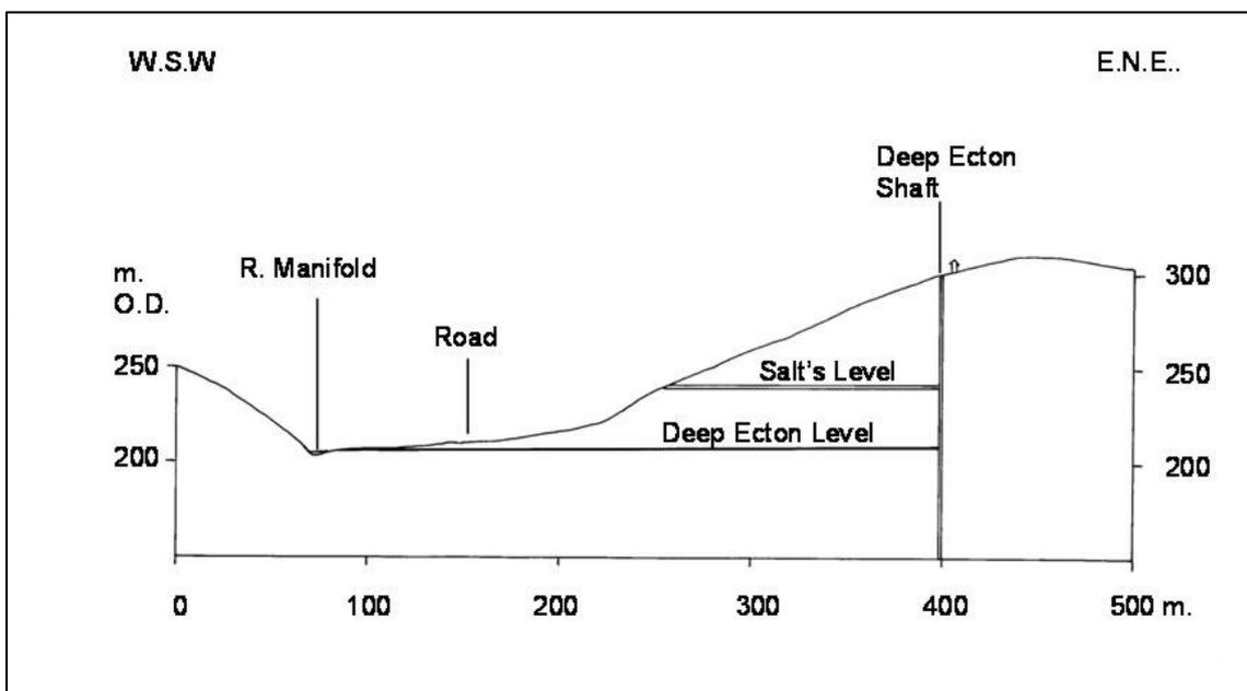
Fig 3.3 Section of Ecton Hill through Salt's Level (natural scale)
